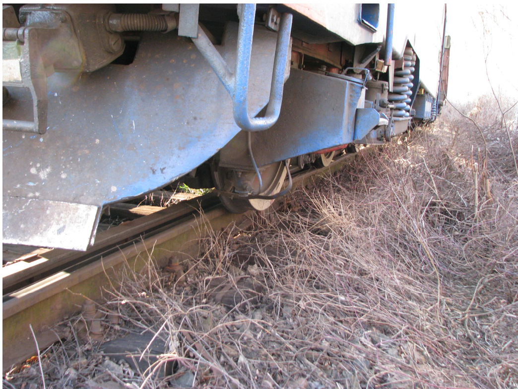
Photo 2 : Locomotive EA 40-0499-0 - derailed
