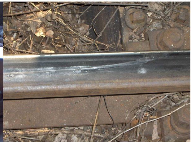
Photo 4: the place of escalating the wheel
